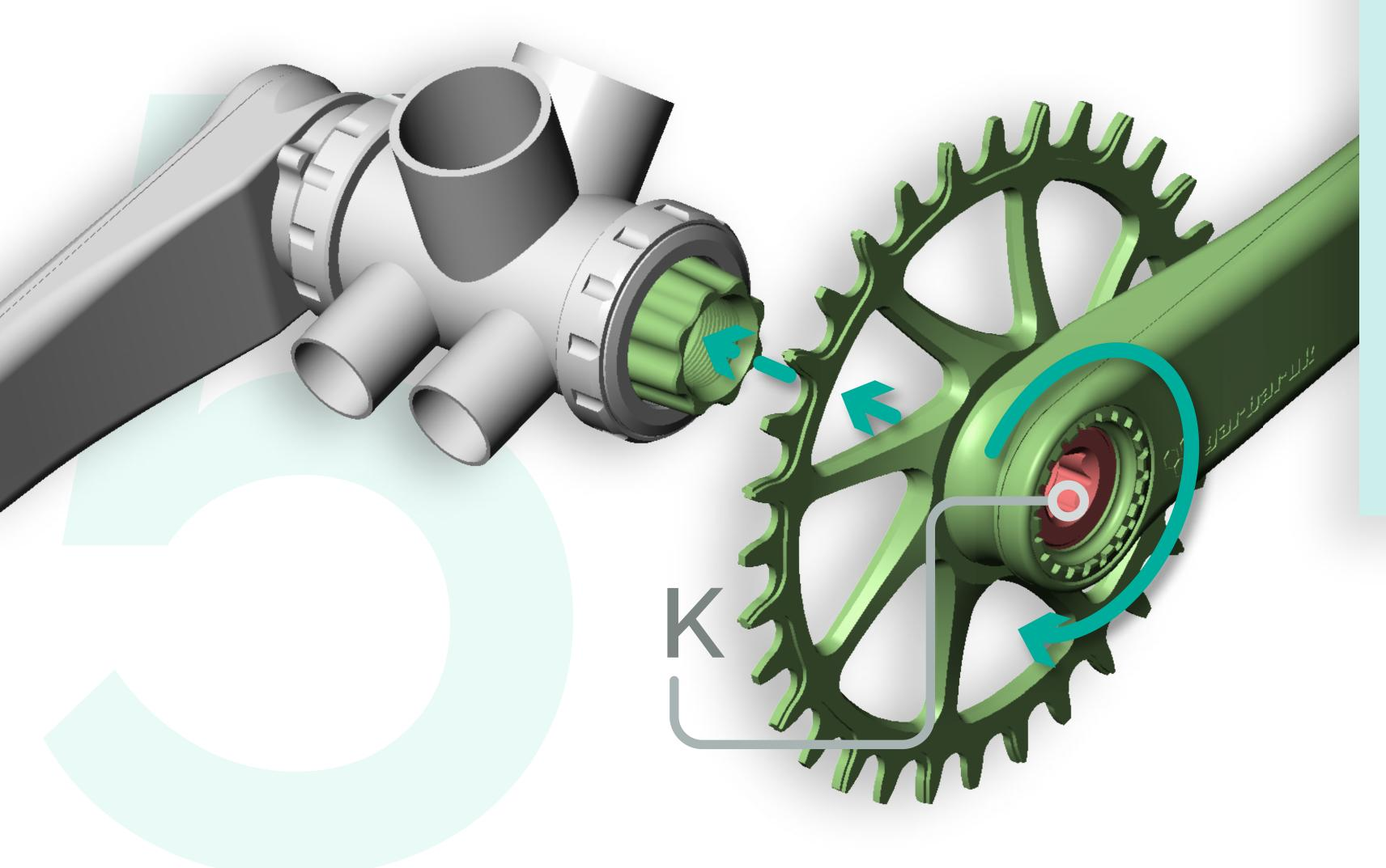
Mount the driveside crankarm. Secure by tightening the crankset bolt (K) with a 10mm HEX key.
