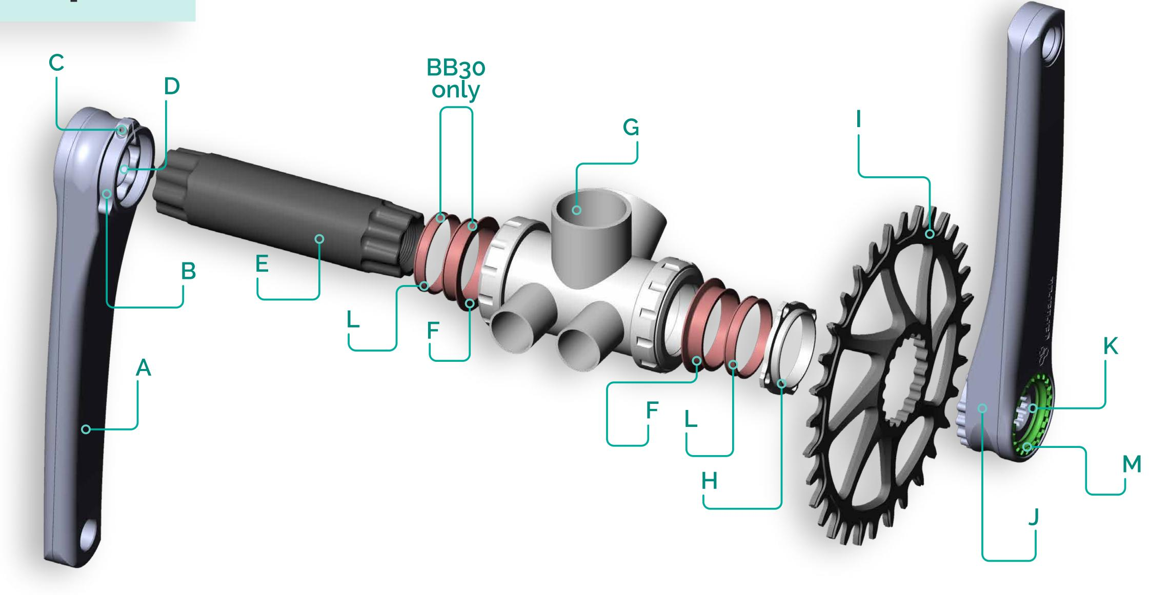
On the non-driveside crankarm, turn the preload adjuster (B) until it gently touches the crankarm (A).
