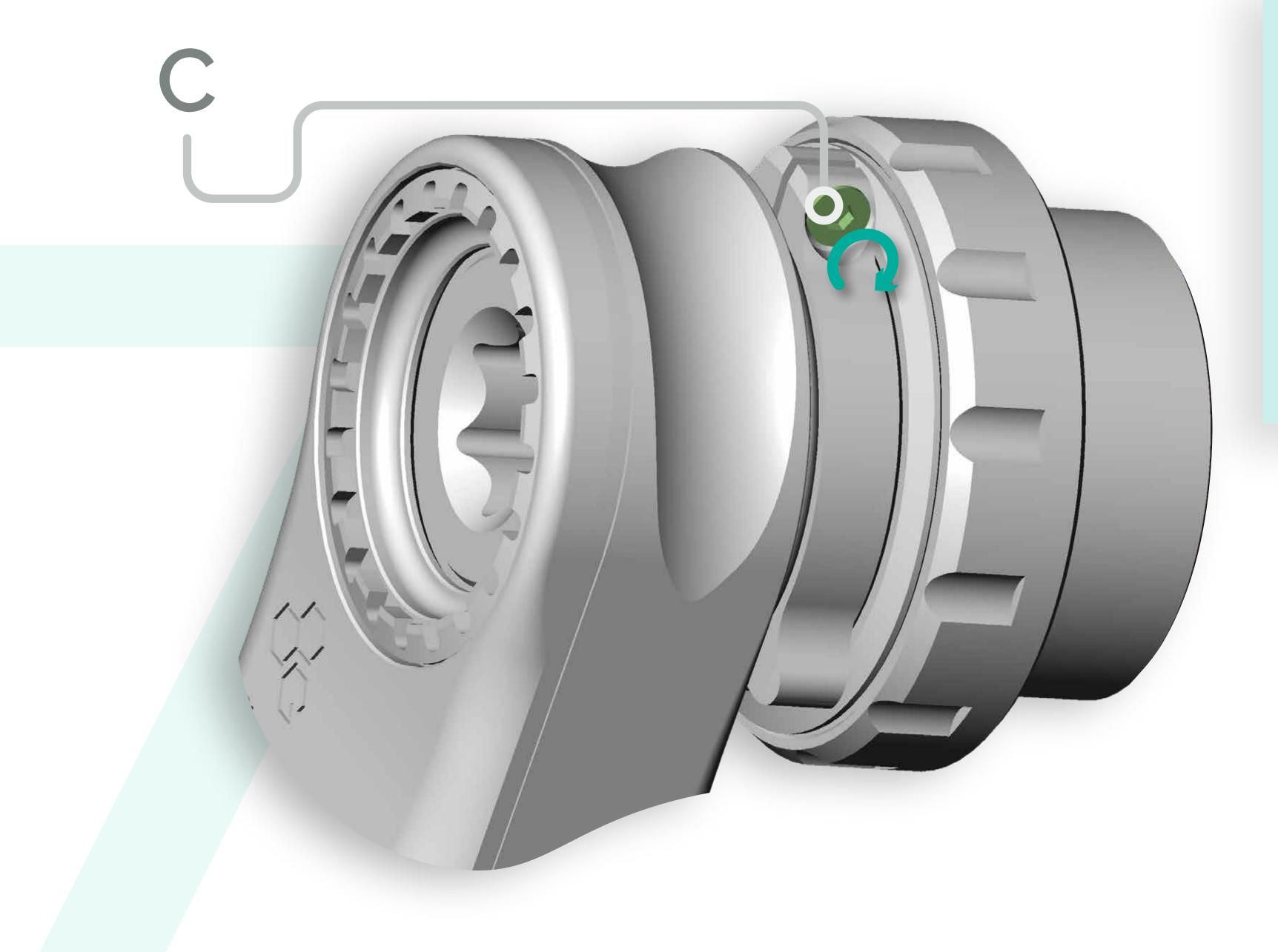
Tighten the securing bolt (C) on the preload adjuster by using a 2mm HEX key. Recommended tightening torque: 1-1.5Nm.
