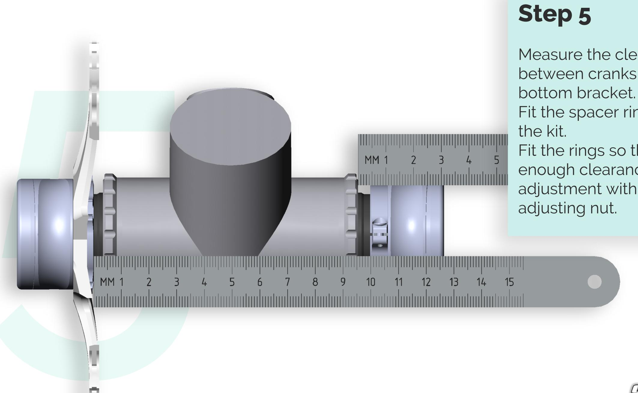
Measure the clearance between cranks and Fit the spacer rings from
