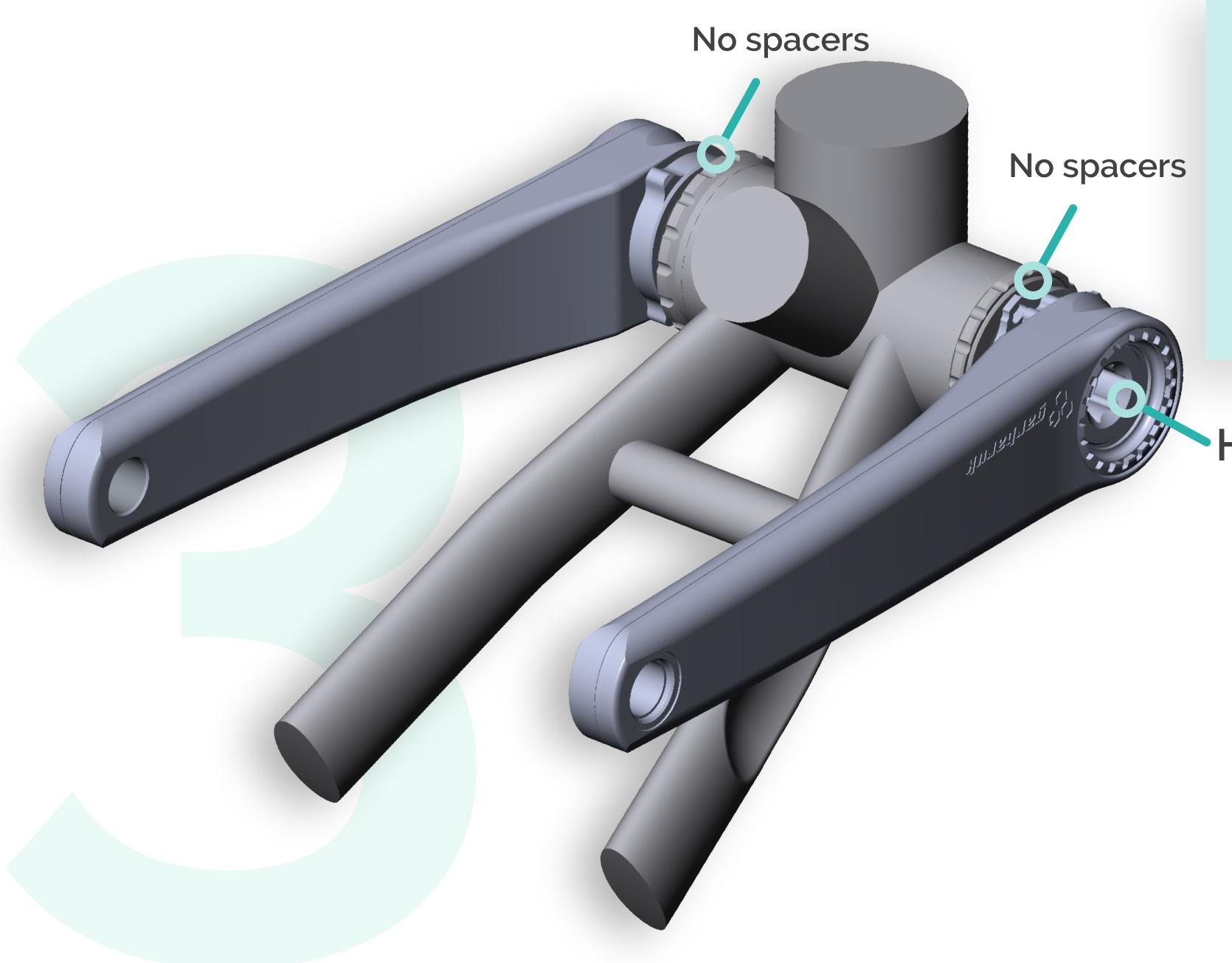
Install cranks in the same direction and tighten the bolts with a torque of 50n/m. Do not install spacers.
